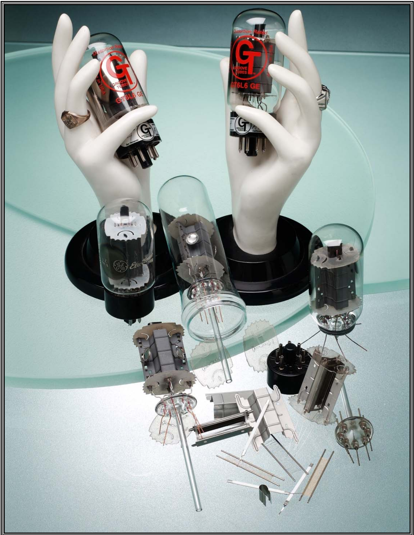
These are components of the new Grove Tubes GT6L6GE, a faithful reproduction of the original General Electric “clear top” tube made on the original GE machines and with many original materials. The various stages of production are pictured here, and an original GE6L6 is also pictured under the left hand that is holding one of the new matched GT6L6GE tubes.
